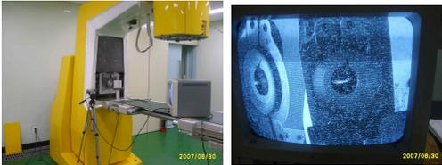
(A) System setup scene of temporary target for measuring beam current and CCD camera for monitoring beam shape.
