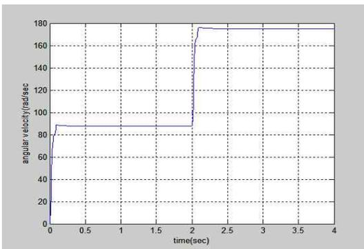
Fig. 3. The plot of angular velocity of rewind roll with proposed method
