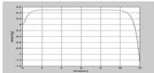
Fig. 5. The plot of tension of web with linearization at  $w_r = 87.5$  rad/sec
